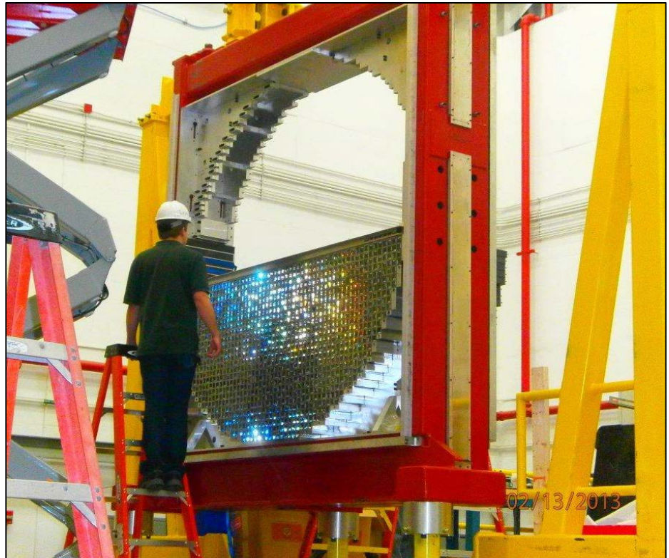
The Forward Calorimeter (FCAL) being assembled in the newly constructed Experimental Hall D.
